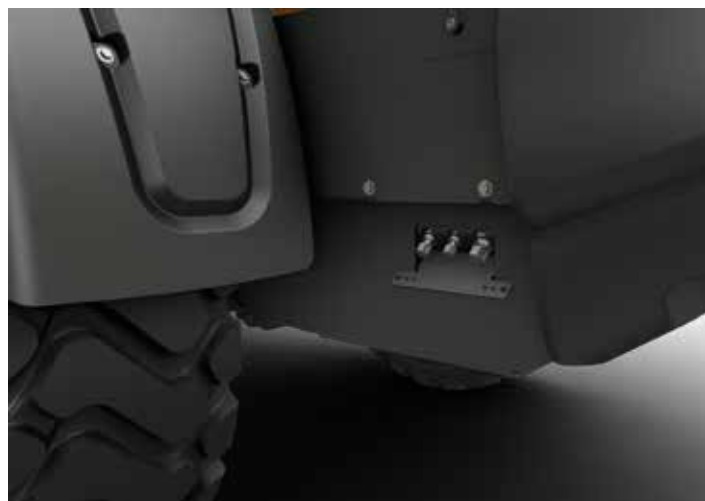
Grouped drains for clean and quick oil changes
